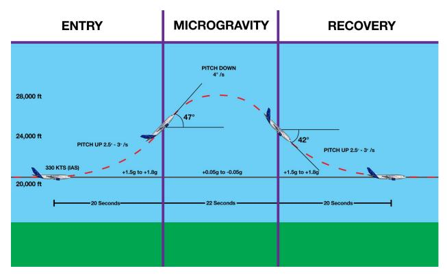
Before initiating the zero-g parabola, the aircraft should be straight and level at 20,000ft, VMO-10 KTS (approx. 330 KTS), in clean configuration. It is recommended to have the flight directors in ALT HLD and HDG modes, and ATHR on throughout. Engine start selector should be in CONT RELIGHT.
