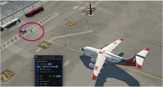
6) After the countdown, **the marshaller will call « Stop »**. When the marshalling hand-pads lights turn red, you have reached your captured parking position.
